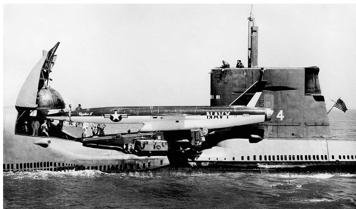
USS Grayback (SSG-574) - one of the first of the Navy's guided missile submarines to carry sea-to-surface missiles. In 1968 the missile chambers were converted to carry 67 embarked troops and SEAL Swimmer Delivery Vehicles (SDVs), including a decompression chamber.
